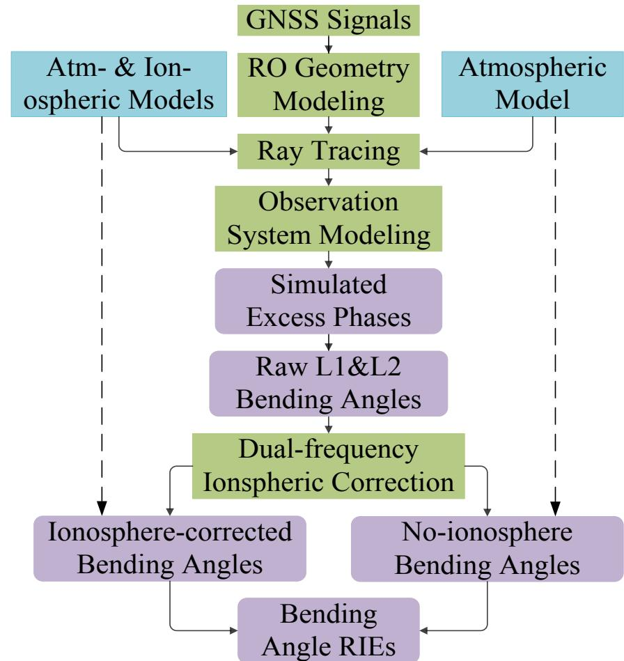
Flow chart of the RO end-to-end simulation process for bending angle RIEs
