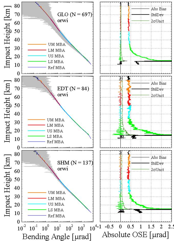
**Ionosphere-corrected bending angle profiles and their statistical results for the 'orwi' dataset.**
