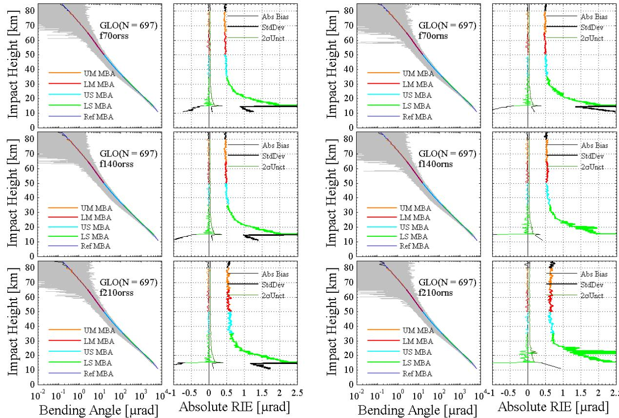
Ionosphere-corrected bending angle profiles and their statistical results for the GLO 'orss' (left) and 'orn' (right) datasets.
