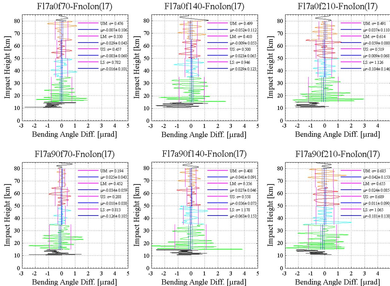
**Absolute RIE profiles of the simulated bending angles and their statistical results over four characteristic height layers, lower stratosphere 15–35 km (LS), upper stratosphere 35–50 km (US), lower mesosphere 50–65 km (LM), and upper mesosphere 65–80 km (UM). (Morning/7:00LT RO events)**
