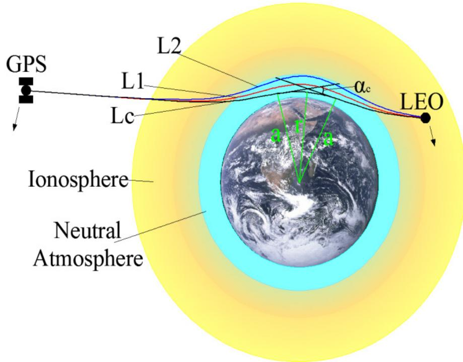
Radio occultation geometry illustrating the separated L1 and L2 signal paths and the ionosphere-corrected ray path Lc
