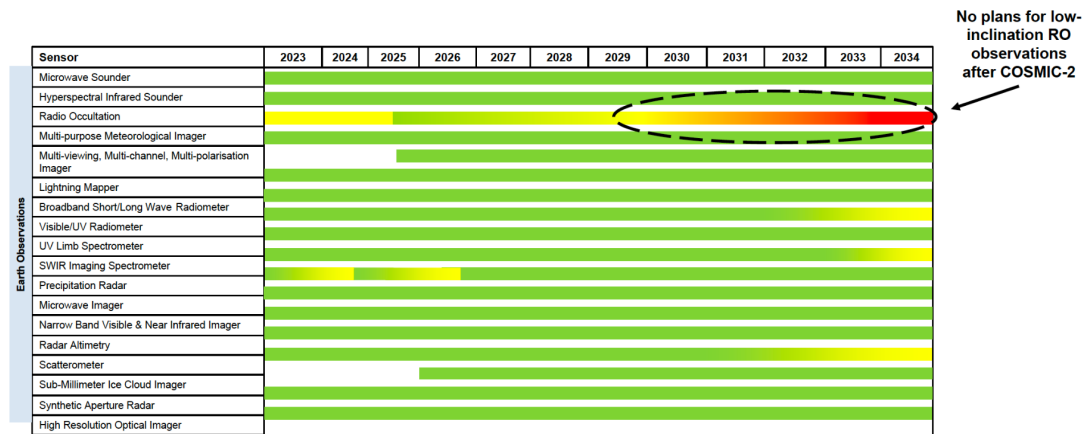
Figure 3: Top level risk assessment of Earth Observations. The risk is highest for radio occultation observations. (A. Mehta, CGMS WGIII report, 2023)
