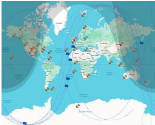
Yunyao data coverage for neutral atmosphere (atmprf, ~33000/day) and ionosphere (ionprf, ~17000/day)
